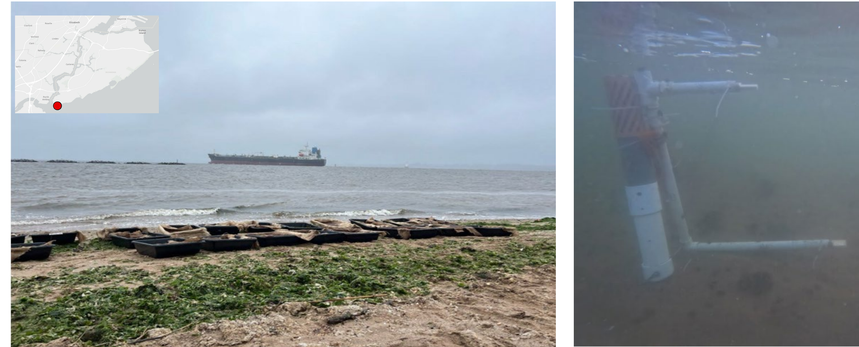
Figure 1. (Left) Eelgrass/shoots/sods ready for planting with the Living Breakwaters in the background. The inset map in the top-left corner shows the general location of the site. (Right) Helical anchor with HOB0 MX801 Data Logger attached on the left, and two HOB0 Pendant Temperature/Light Loggers attached on the right via a PVC structure that maintains a set distance between the two pendants.
