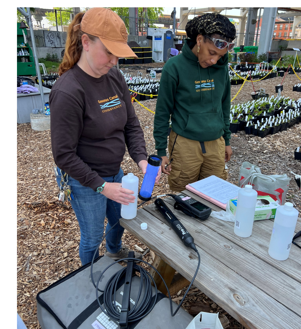
Jennifer Kepler and Aurelia Casey learning how to calibrate the YSI ProDSS multiparameter water quality meter.
