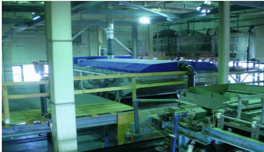
NEWLY INSTALLED BELT FILTER PRESS
