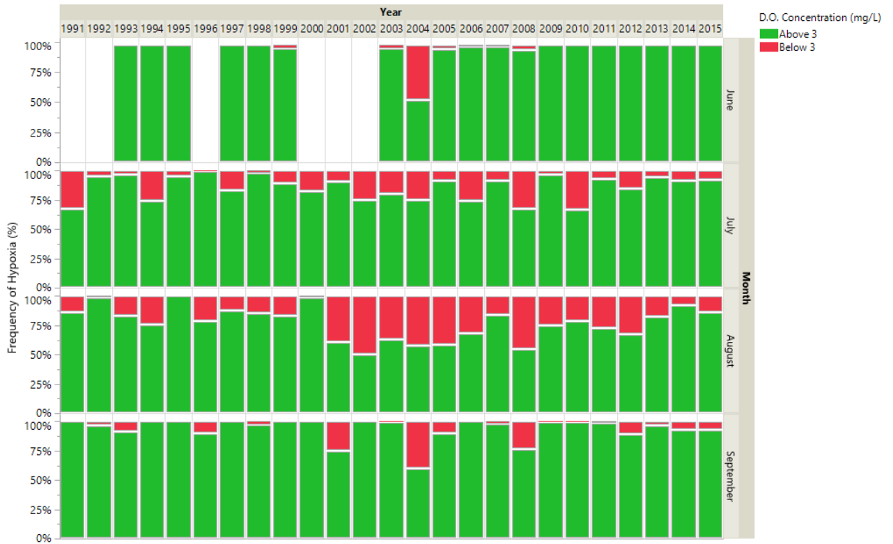
EXHIBIT 5-4 FREQUENCY AND DURATION OF HYPOXIA: PERCENT OF ALL SAMPLES BY YEAR AND MONTH ABOVE AND BELOW HYPOXIC CONDITIONS (3 MG/L).
