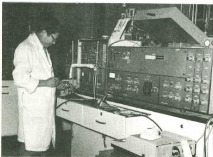
Gas Chromatograph. This unit is used for the analysis of many parameters, including benzene, PCB's and pesticides.
