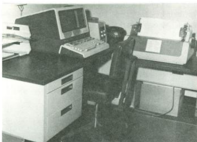
Data Processing. CRT terminal with dual tape cartridges, a printer and a multi-speed modem. This system is used to communicate with time share computers and with state and federal agencies.
