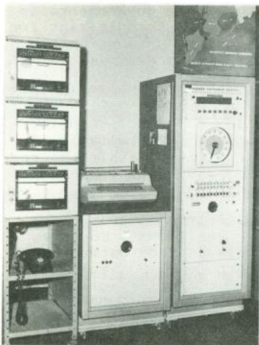
Telemetry Receiving Units. Central receivers for remote instrumentation located throughout the Interstate Sanitation District. Three wind speed and wind direction receivers are shown on the left. The receiving unit for the remote automatic water quality monitoring system is shown center and right. This unit produces a printout of the data and punches a paper tape for computer processing.
