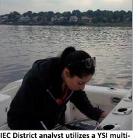
IEC District analyst utilizes a YSI multiparameter meter to measure the *in situ* parameters at station A2M.
