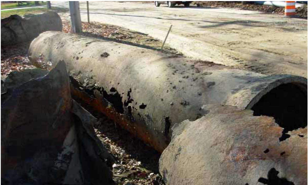
Corroded 25-year Old Ductile Iron Gravity Sewer Photo Courtesy of Milford-Housatonic WPCF
